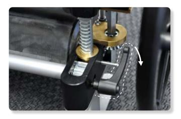
4. Secure the height using the lever on the side of the press. (see picture)
