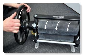
6. Feed your liner through the roller by winding the operating wheel. (see picture)
