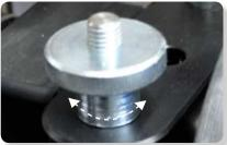
5. You can limit the maximum opening by adjusting the securing nuts on top of the roller. (see picture)
