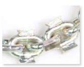
Thoroughly check the chain to verify that it is in good condition and that the carbide tips have not significantly worn off.
