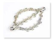
Based on job demand, choose the correct chain size. The right size of chain can be determined by the diameter of the pipe you are about to clean with +25%.
