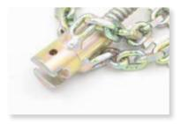
1. Check out that t-slide connectors are clean and the male connectors nob is moving (grease, if it's necessary).
