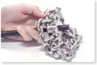
2. When attaching the chain, make sure that there's around 10mm of bare shaft / cable over at the end so that the screws can be properly secured.\*
