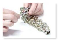
1. Loosen the screws on both sockets on the chain. Bring the shaft / cable through both sockets.
