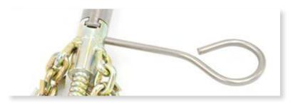
**3.** Detach tool by pushing T-slide opener key RA-014 or RA-015 through a hole on the connector.
