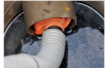
The pipe will automatically be sealed airtight as soon as smoke passes through the hose
