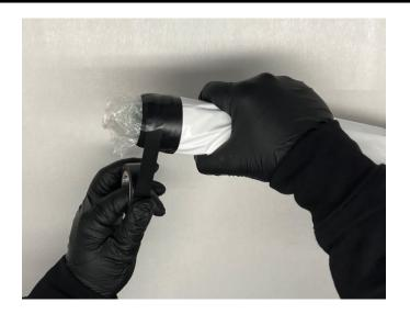
Secure the support hose in position by taping it to both end caps. Do not cover the threaded connectors on the end caps.
