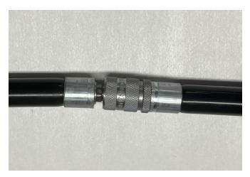
To join the rods together you align the hex socket, push fittings together and then tighten the locking ring.
