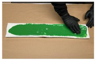
Apply resin in portions and work it thoroughly into the material.
