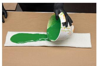
After resin is mixed according to the instructions, pour a portion on the surface of the material.
