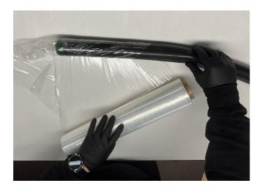
**Before** covering the Bendy Packer with the stretch film, attach pull ropes etc.
