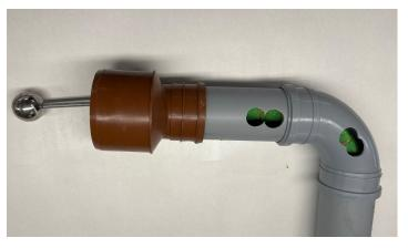
Navigate the Packer until you meet the tape marks on your Push Rods. The Packer should now be on the renovation location if you have accurately marked the correct distance to your Push Rods. Use an inspection camera to check that the Packer is properly positioned.
