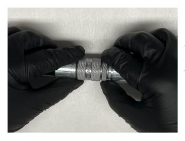
The Picote Push Rods have to be secured with the locking ring, which is located on the rear of the female-type fitting.
