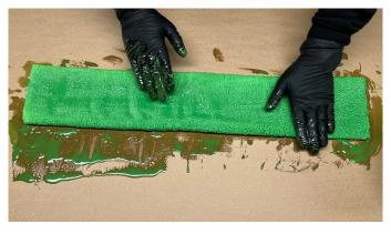
Secure that patch is properly impregnated & resin has absorbed evenly.
