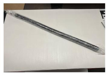
Ensure that the whole length of the Bendy Packer is covered with the film.
