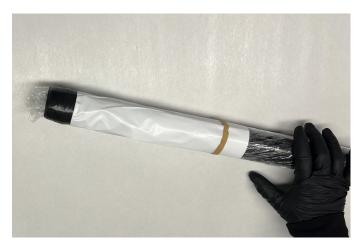
Secure the supporting hose by taping it to the metal end cap and use a doubled over rubber band at the far end of the support hose.
