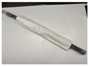
Cut the required amount of liner/patch staying within the section between the off-limit-zones.
