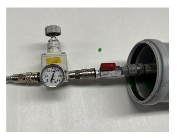
Inflate the Bendy Packer using a pressure regulator until it has reached its operating pressure.
