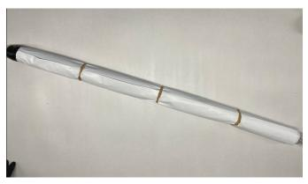
Finally, use rubber bands (doubled over if needed), approximately every 25cm (10"), to secure the support hose on to the bladder.
