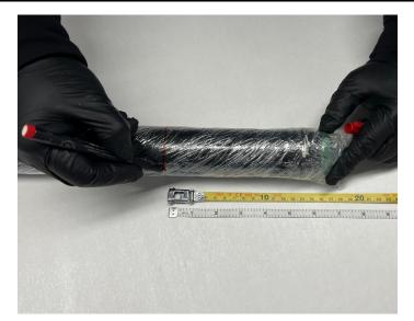
Check the off-limits-zone from the table on Page16, measure the distance on the on the surface of the film using a suitable marker pen.
