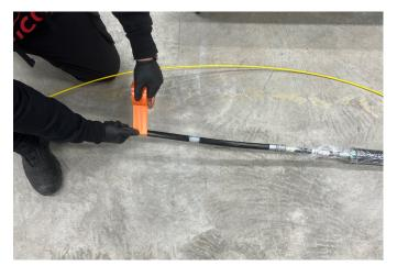
Using the marker tape on the camera as a guide, fasten another piece of PVC marking tape onto the Picote Push Rod to indicate the correct distance to install the repair in the pipe.
