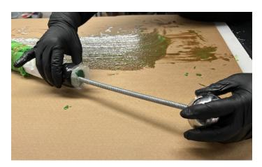
Depending on job site: Install Navigation Guide Ball or Pull Rope to the connector on the end cap if needed.
