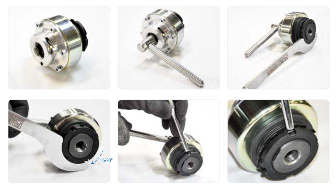
Adjust the torque by tightening or loosening the nut.
